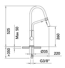
3-way semi-professional sink mixer for water treatment equipment with 2 water outlets, 2 additional spray functions, swivel spout and flexible hoses 3/8" >350mm.
